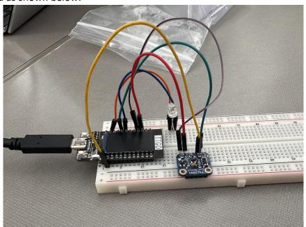
Through this testing, we were able to get the LED to turn off and on as well as read in information captured by the PD. This tells us that the components we are working with are functionally able to complete the task for our project and could potentially work for our PCB implementation of the project as well.
